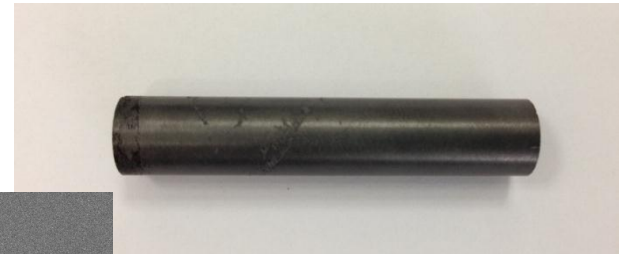
Triplex composite tube (surface machined)
